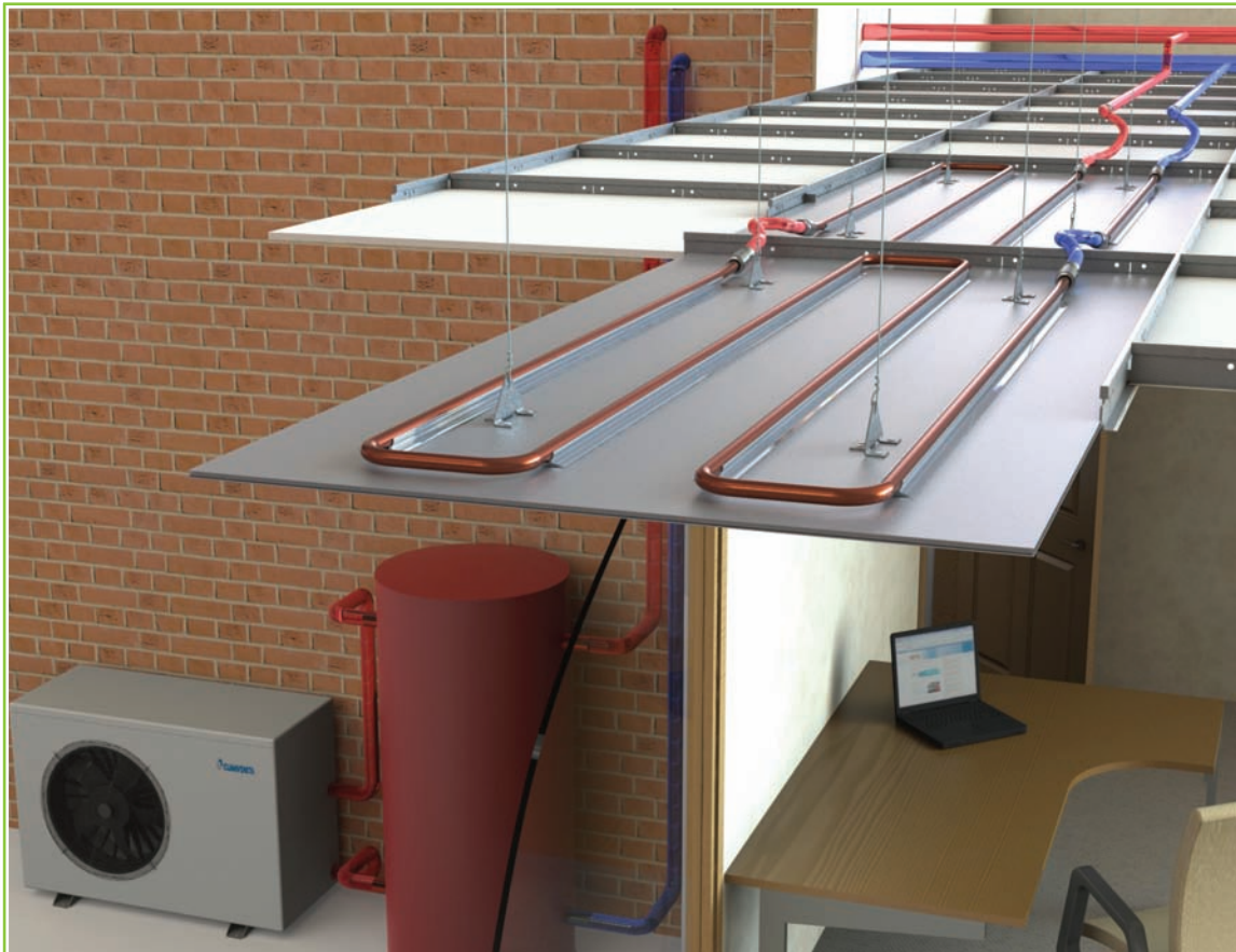
Scematic of a typical installation
