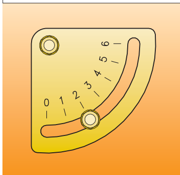
Example of air damper of GI/EMME burners
